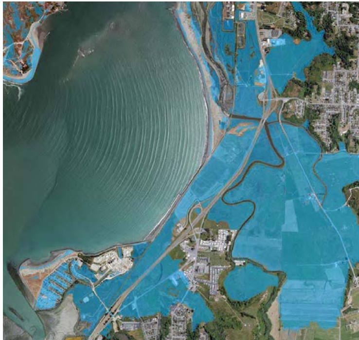
Figure Climate-6. Middle segment, South of Eureka existing conditions: Assuming tidal elevation is 9.99 feet (MMMW+100- year stillwater level) and that protective shoreline structures are compromised, the land adjacent to the road prism is flooded to the west and east of Highway 101, with limited flooding of south and north bound lanes. Source: Laird 2015 (Figure 23)
