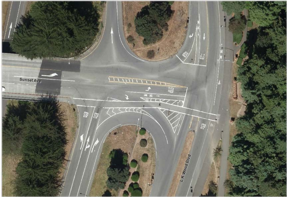
Figure 2.1 The current configuration of the two intersections located within the project area. The Sunset Avenue/US 101 northbound ramp intersection is a four-legged intersection with the north and south leg acting as US 101 Northbound on- and off- ramps. The Sunset Avenue/LK Wood Boulevard is an all-way stop located 150 feet east of the Sunset Ave/US 101 northbound ramp intersection.
