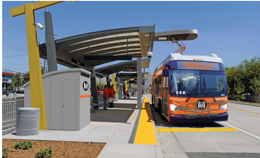
Figure 5: Example mock-up image of a high power on-route charger integrated with a transit stop. Image from energized.edison.com.
