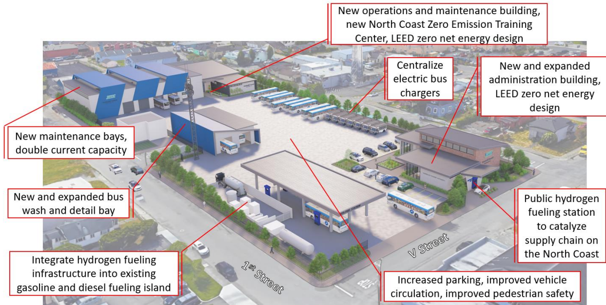
Figure 5: Early draft concept of a redesign and replacement of HTA's existing Administration and Maintenance Facility.
