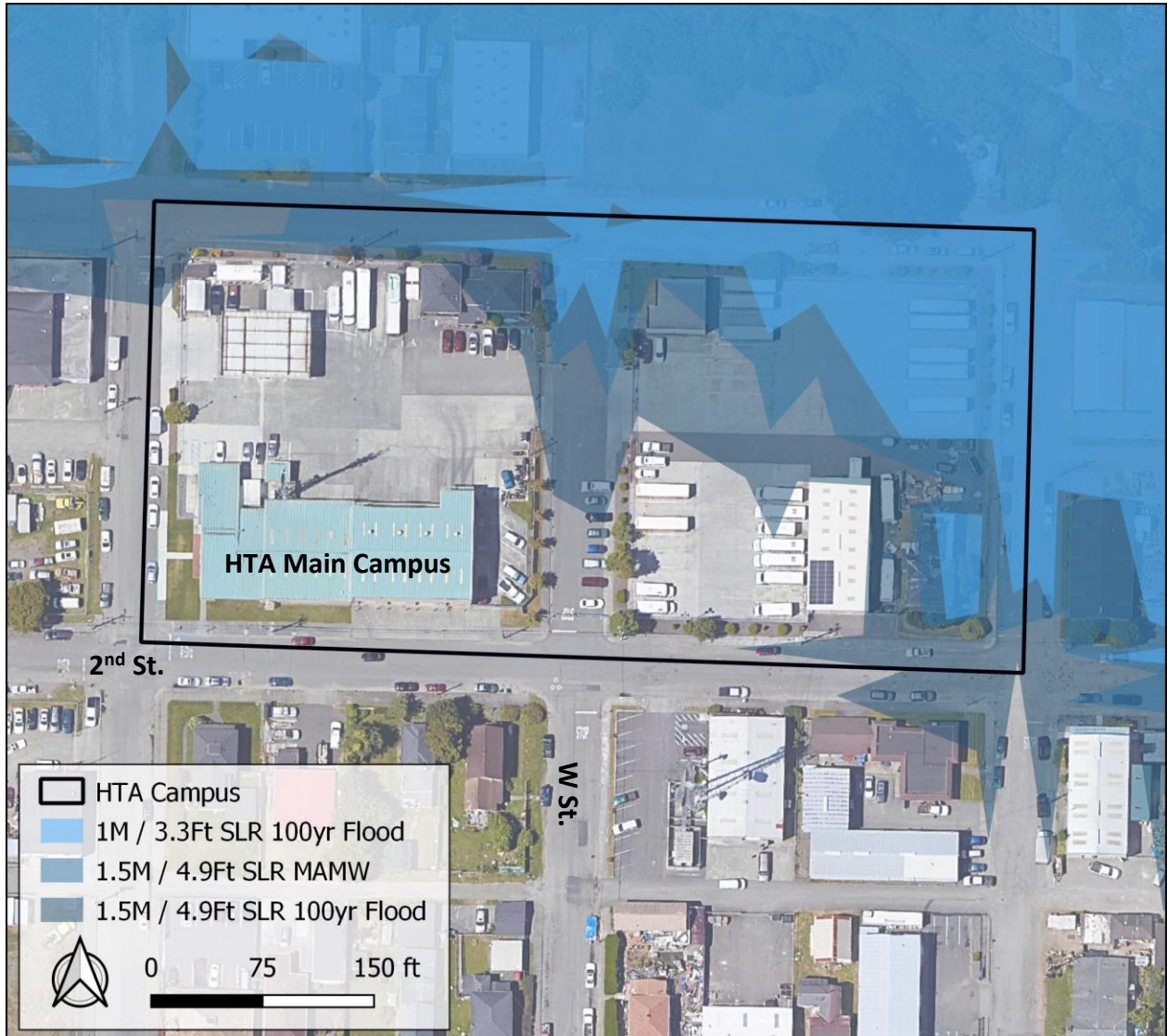
Figure 9: Flooding at HTA campus under 1-meter (2070 high projection) and 1.5 meters (between 2070 and 2100 high projections) sea level rise scenarios. Note mean annual maximum water (MAMW) layer indicates areas that have a high likelihood of annual inundations. Created by the Schatz Energy Research Center. Source: Google Satellite Map, Northern Hydrology and Engineering (2014b).
