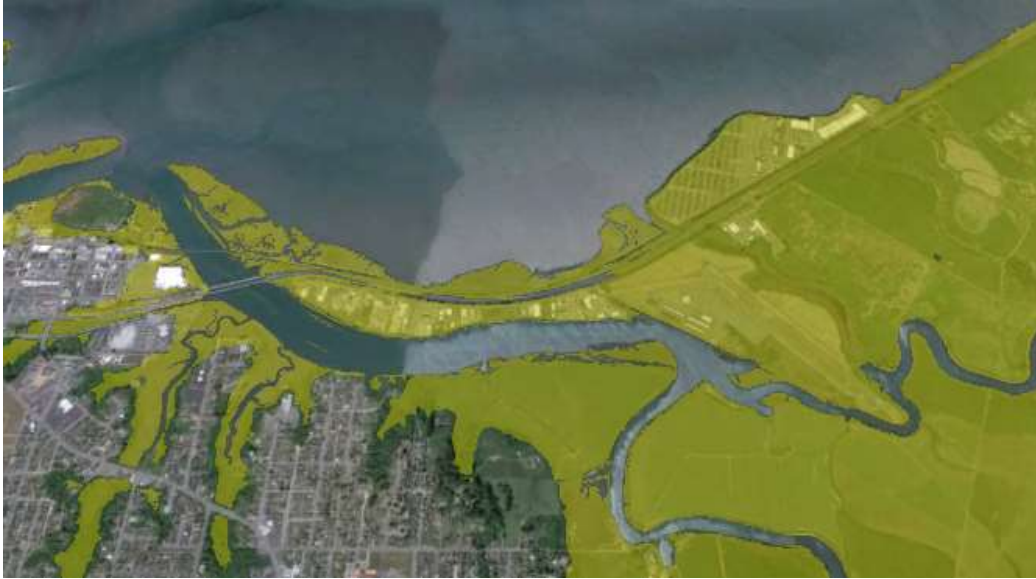
Figure Climate-7. US 101 Eureka to State Route 255 Possible Inundation Inundation map of northeastern Eureka and Highway 101 with a half-meter of sea-level rise, which is predicted for the year 2050. Source: NHE 2015
