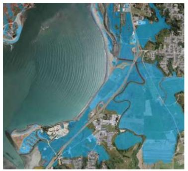
Assuming tidal elevation is 9.99 feet (MMMW+100-year stillwater level) and that protective shoreline structures are compromised, the land adjacent to the road prism is flooded to the west and east of Highway 101, with limited flooding of south and north bound lanes.
