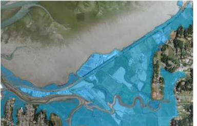
Assuming tidal elevation is 9.99 feet (MMMW+100-year stillwater level) and that protective shoreline structures are compromised north of Airport Road, extensive flooding of south and north bound lanes.
