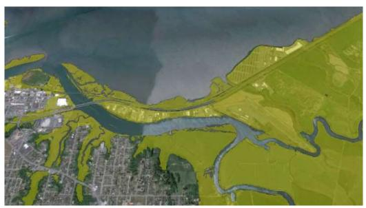
Figure Climate-7. **US 101 Eureka to State Route 255 Possible Inundation** Inundation map of northeastern Eureka and Highway 101 with a half-meter of sea-level rise, which is predicted for the year 2050. Source: NHE 2015
